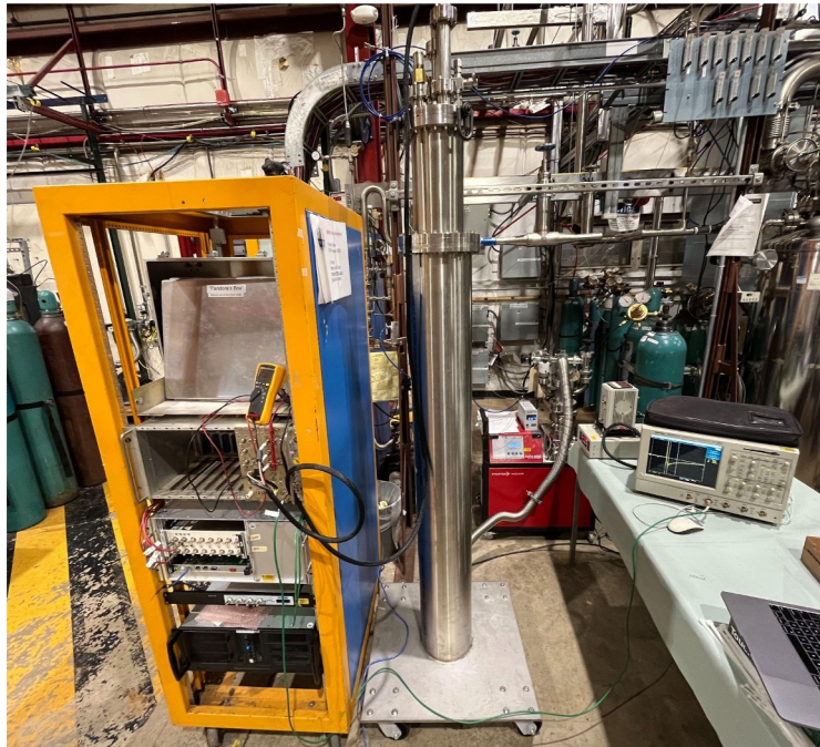
Purity Monitor Test Setup at NLTF
