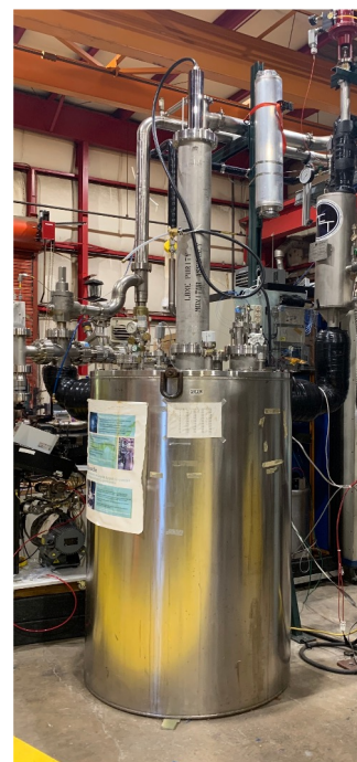
HV FT Test Setup in BLANCHE @NLTF
