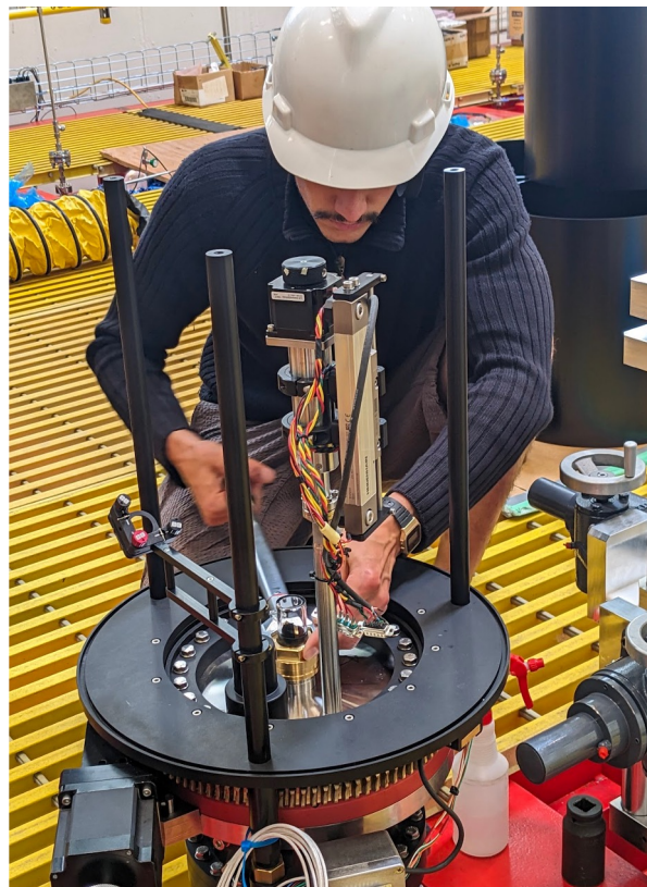
Installation of the four laser feedthroughs on the cryostat
