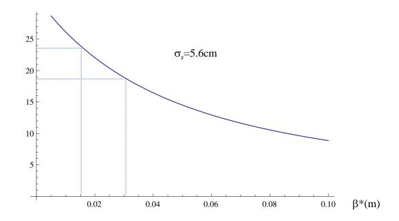
At  $\beta^*=2.5$ cm the hourglass factor = 0.5, the gain in luminosity with  $\beta^* \rightarrow 1.5$ cm is just 17% - still can be worthwhile.
