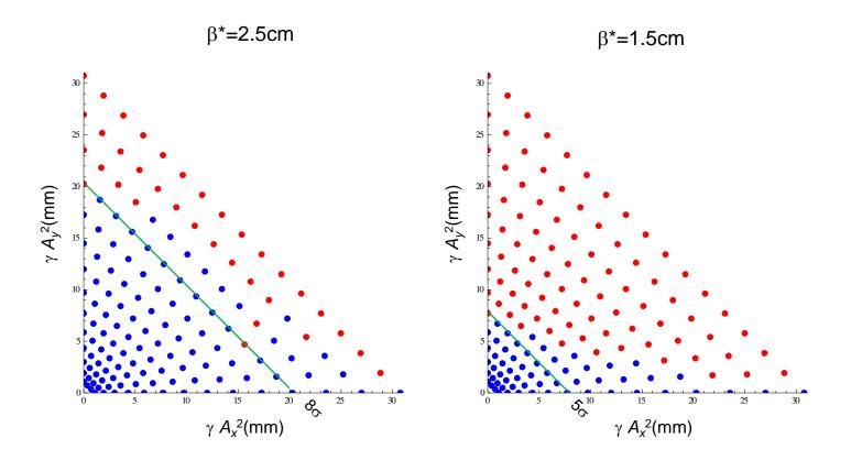
2048 turns Dynamic Aperture (DA) computed with MAD8 LIE4 method. Octupole correctors were used to correct vertical detuning with amplitude. In both cases the DA significantly exceeds the physical aperture ( $5\sigma$  and  $4\sigma$  respectively)
