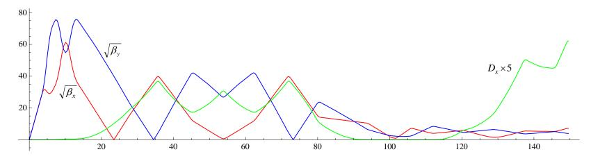
$\beta^*$  can be increased up to 10 cm by changing quad gradients in the matching section
