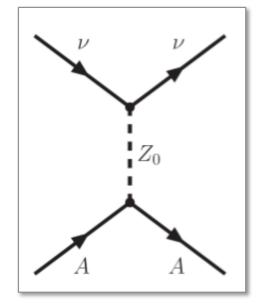
If we can observe coherent neutrino scattering then with either a Ge or Ar based detector.
