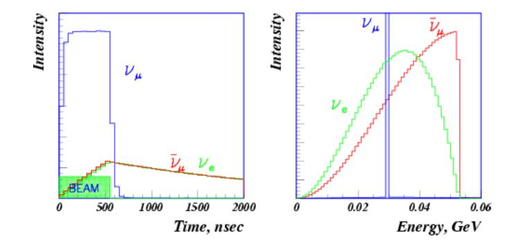
Simple beam dynamics well determined by the kinematics of the pions decaying at rest.
