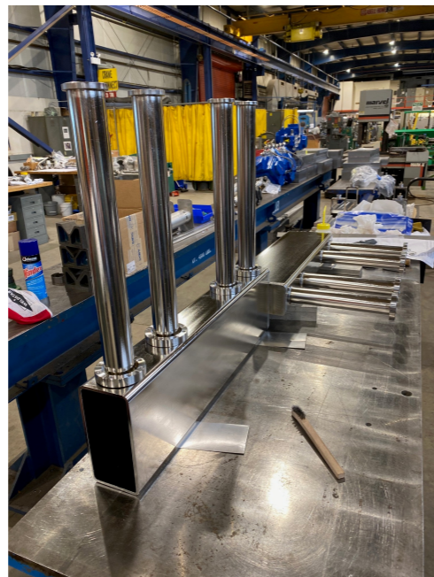
Secondary collimator vacuum chamber
