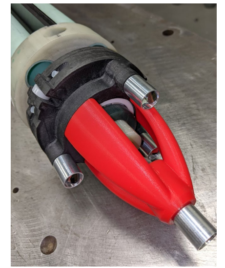
Laser tracker targets visible from non-drive end
