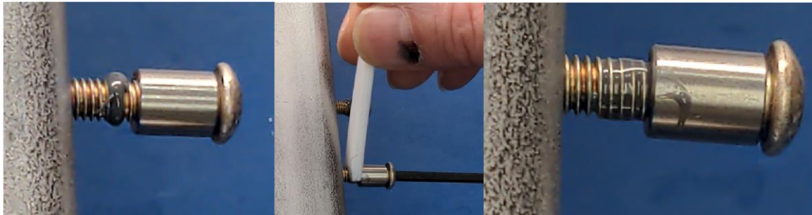
Figure 2 – (left) epoxy just applied to M4 screw. (Centre) using tool to press epoxy into threads. (Right) epoxy in threads, ready for installation.
