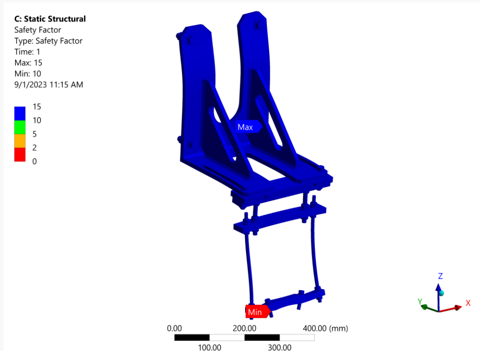
Figure 20 End Flange Holder FEA Safety Factor
