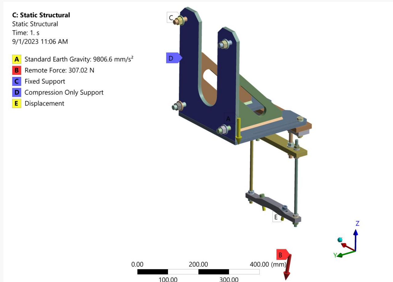
Figure 16 End Flange Holder FEA Boundary Conditions
