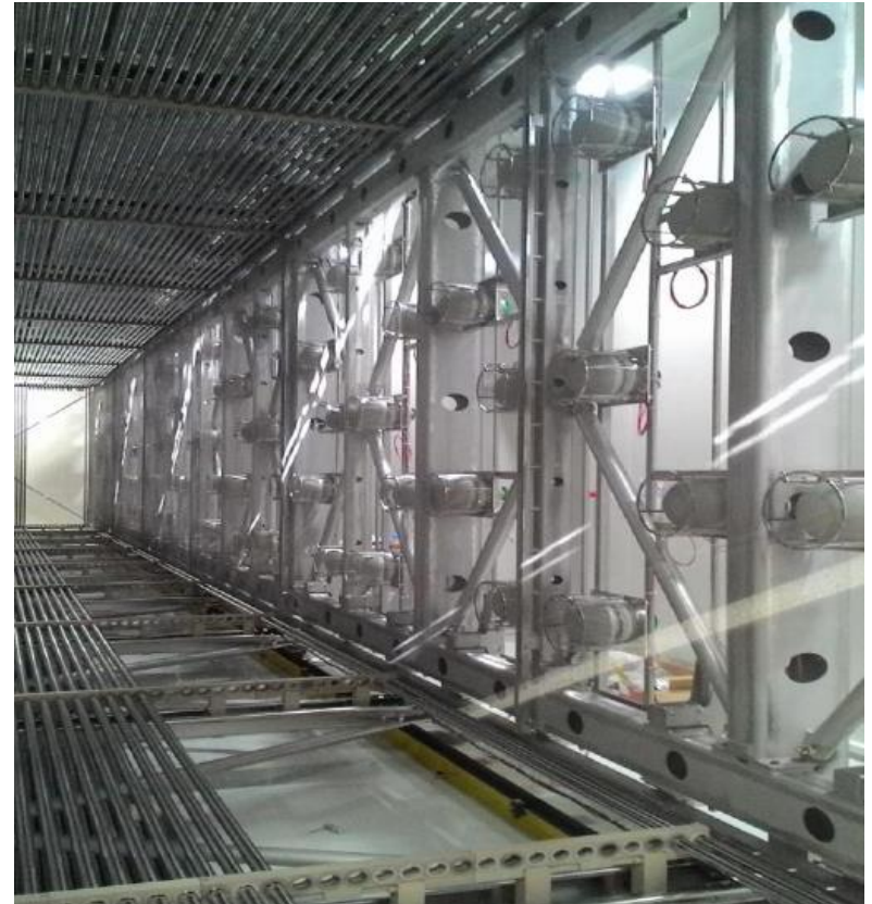
Picture of the insides of an ICARUS TPC; there are 90 PMTs in each TPC
