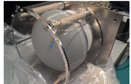
Picture of a PMT on its support with the optical calibration fiber
