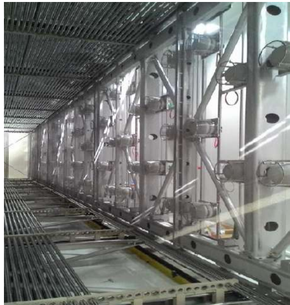
Figure 2: Picture of the PMTs mounted on one of the inner walls of the ICARUS TPC [5].
