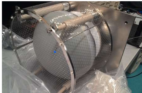
Figure 3: Picture of a PMT in its stainless steel cage and an optical fiber pointing towards it [6].
