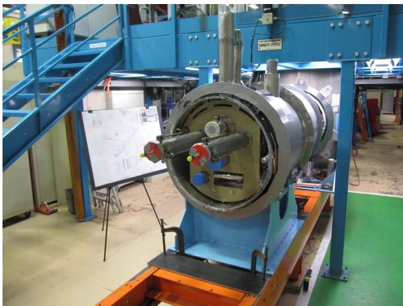
Figure 77: New Adapter Box with a thermal shield between the feed can and the Cryo-Assembly.
