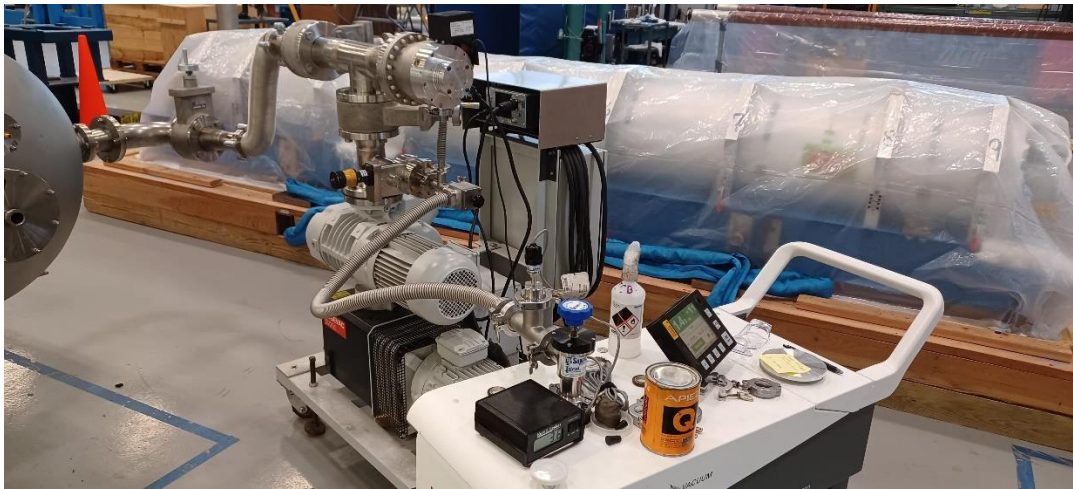
Figure 1 – Pumping cart being backed by Adixen MSLD
