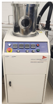
Figure: Parylene coating machine
