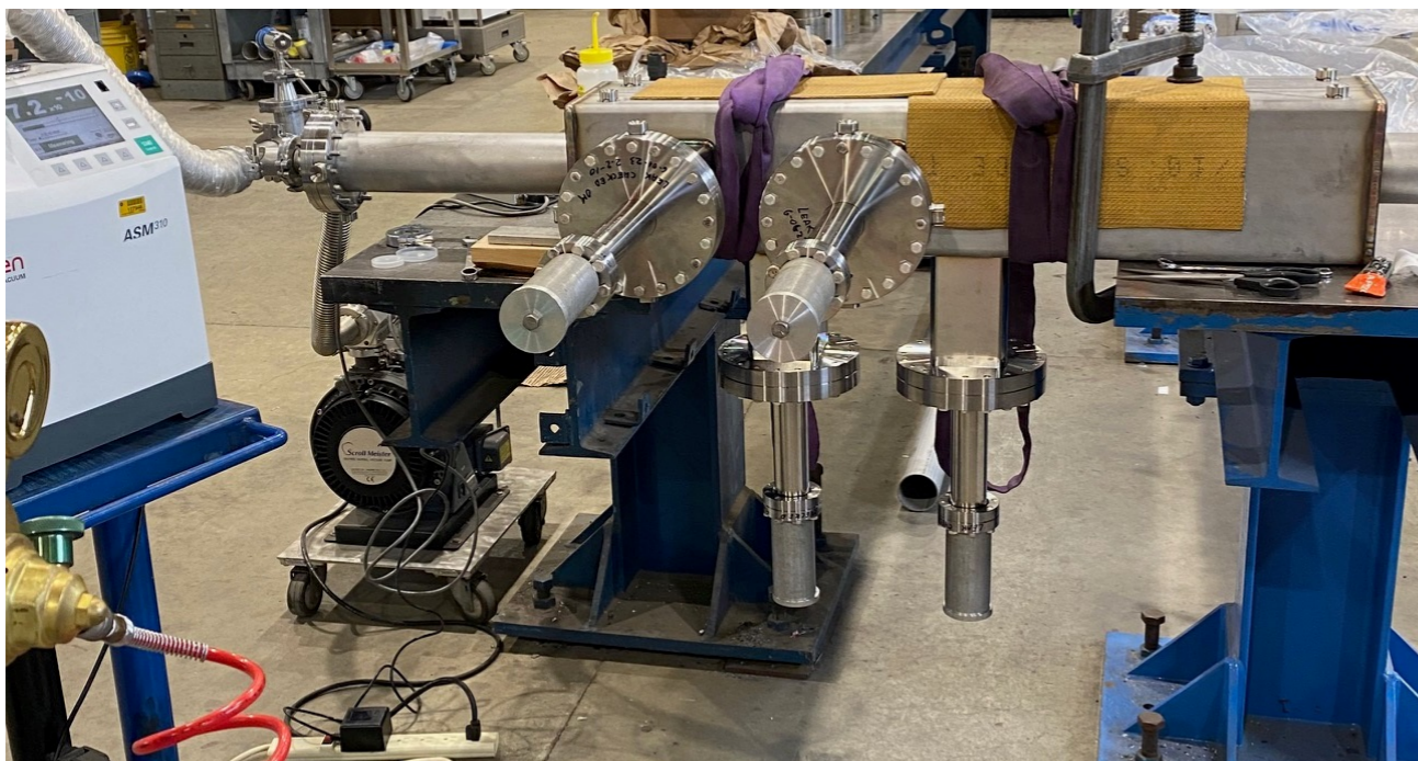
Primary collimator vacuum chamber with jaws inside
