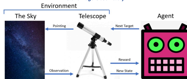
Diagram of the RL setup. A trained agent takes the current state of the sky, and moves the telescope to the next optimal target
