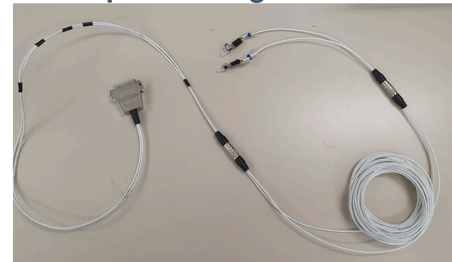
Test passthrough cables
