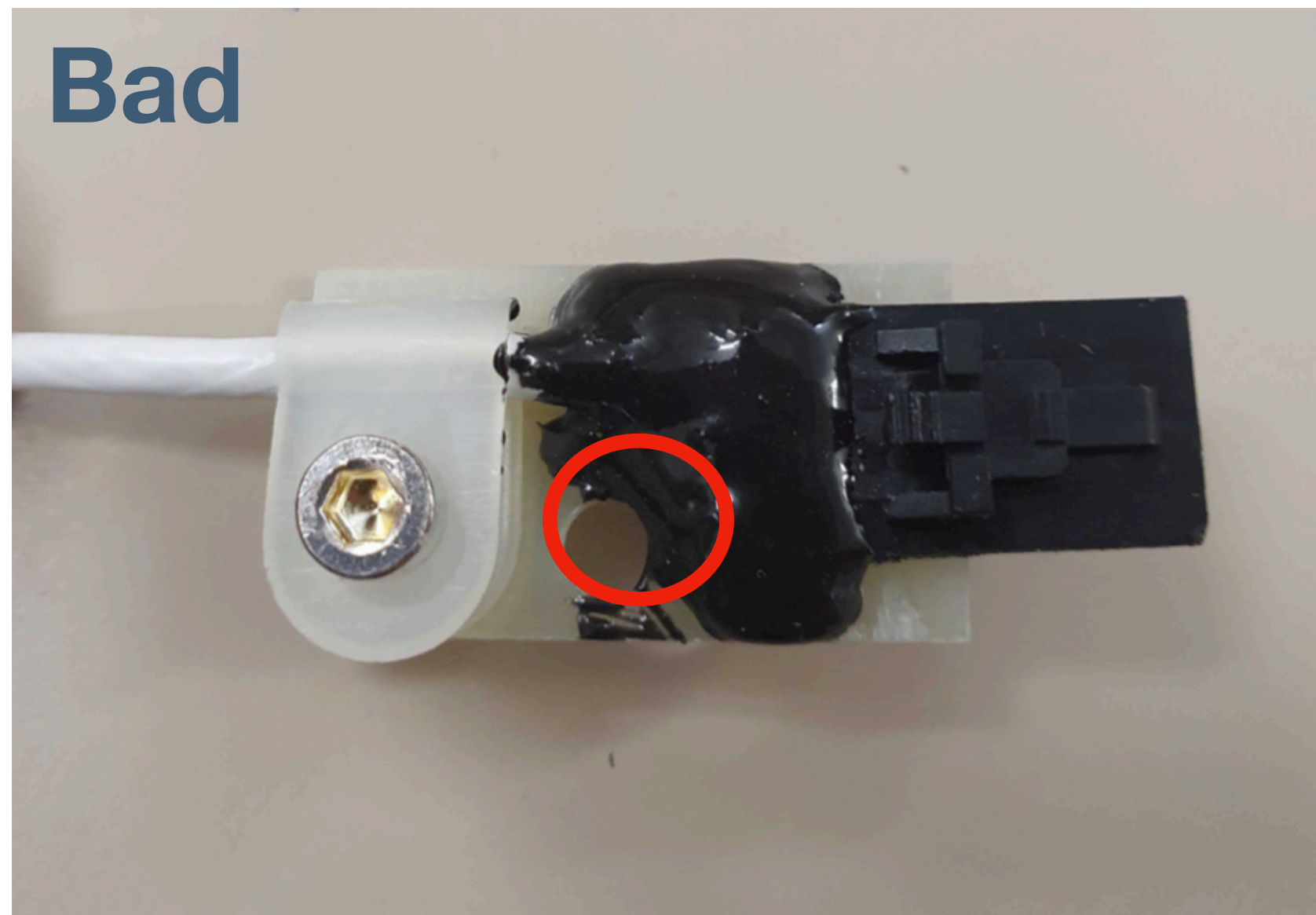
Cable is too close, cannot be easily repaired
