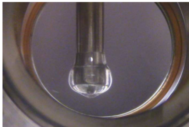
Cryoprobe-based extraction for nEXO
