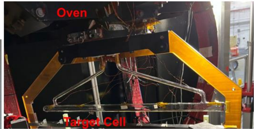
Polarized helium-3 target as effective polarized neutron
