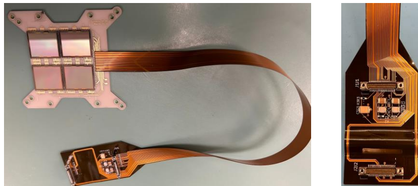
Figure 4. Left: Photo of the sMCM with the GPIO flex cable attached. Right: Closeup of flex cable.
