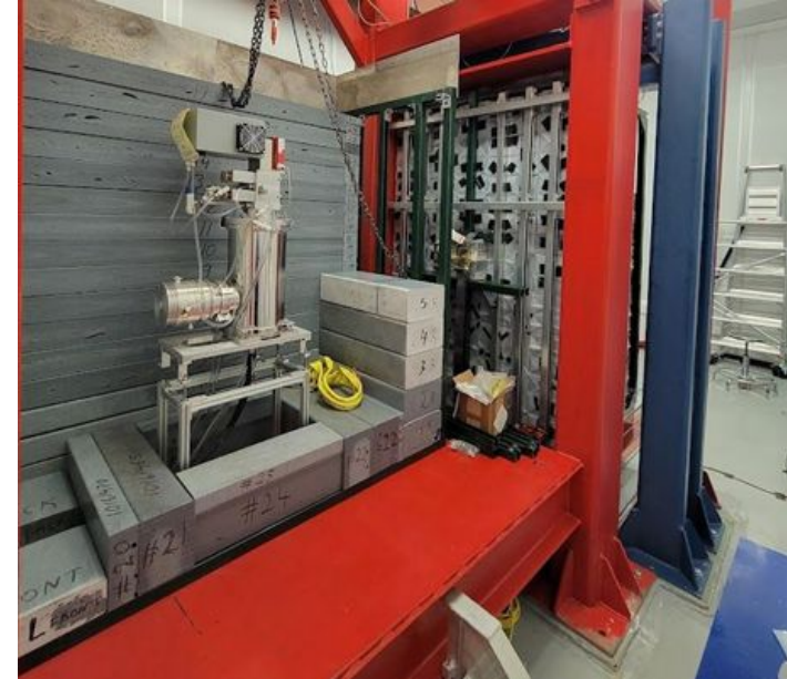
Exposed view of the NEXUS D-D Generator (image courtesy of Dylan Temples)
