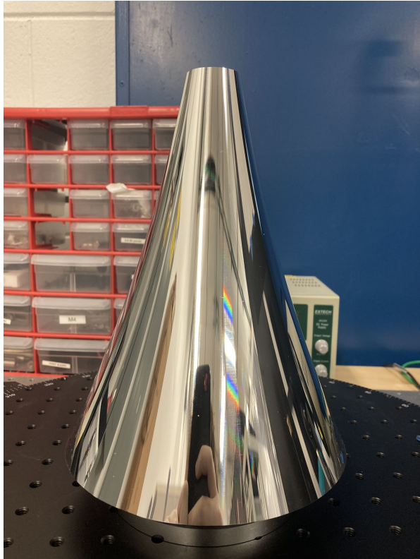
Upper reflector half on the rotating table. Part is centered to the table through the central bore.
