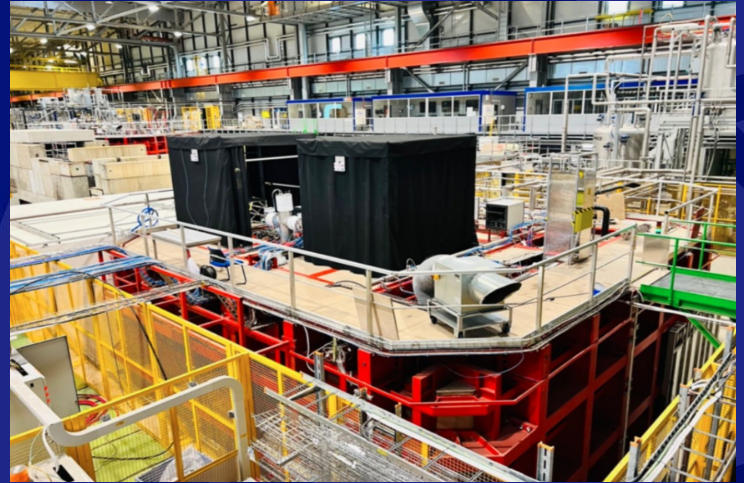
Tents for both laser periscopes (black) sitting on top of the ProtoDUNE cryostat
