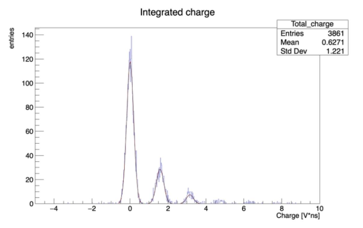
Amplitude max = 1.60723V Range = 1458 rise time 220ns decay time =2636ns undershoot fraction 0.845148 %
