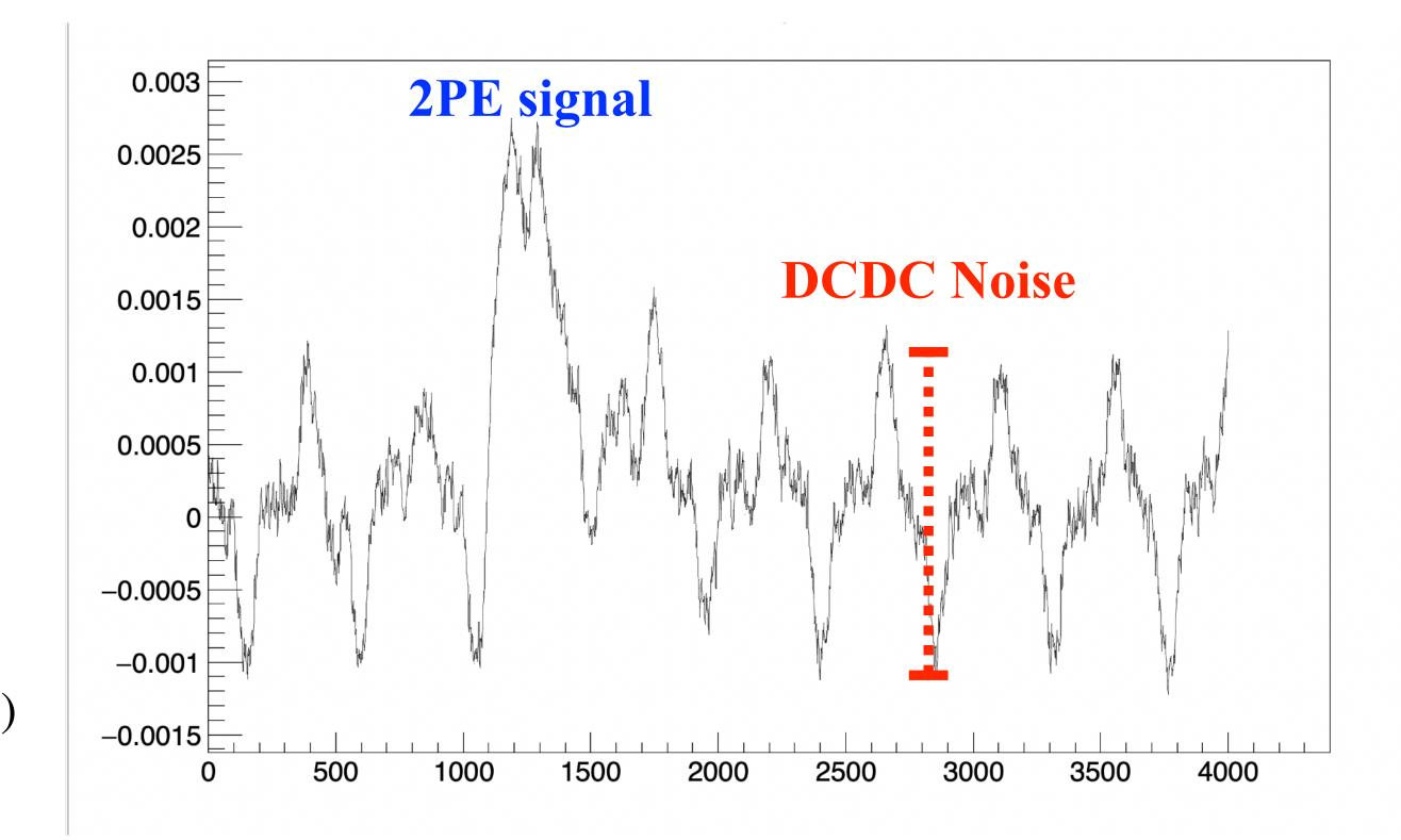
In LAr situation, the noise level is high compared to SPE amplitude:
