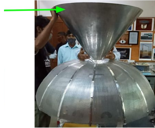
Monocone antenna design on shaped reflector (55 -110 MHz)
