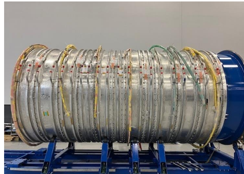
Detector Solenoid in progress
