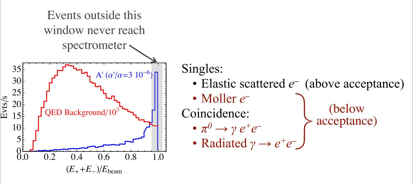
Dominant coincidence background (accidental  $e^{-\pi^+}$ ) can be rejected by using Gas Cherenkov detector in coincidence trigger.<sub>7</sub>
