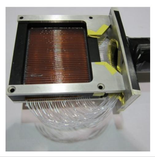
Active "sieve slit": tagging by a Sci Fiber detector
