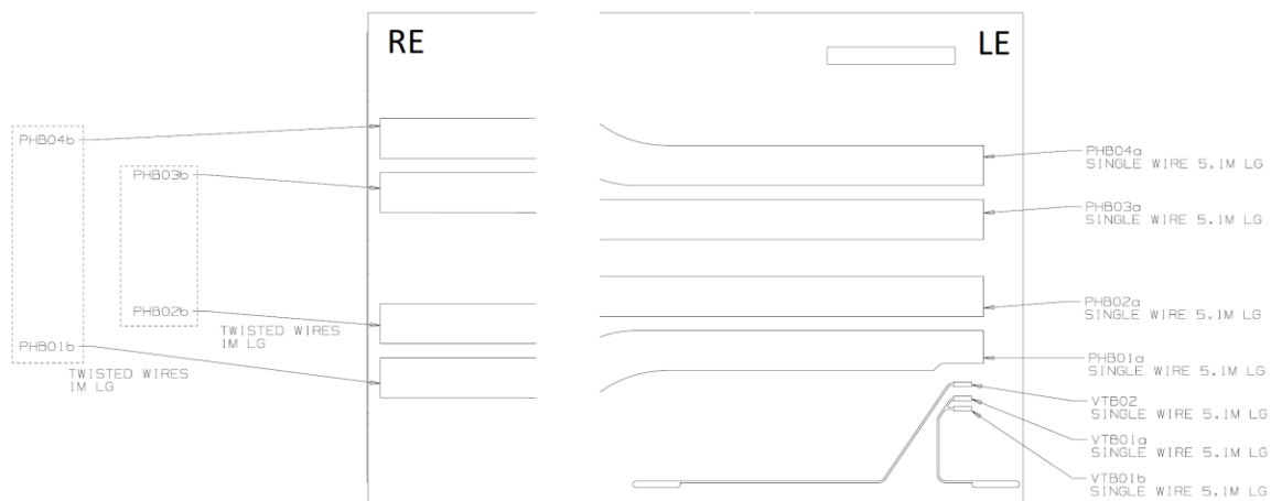
Figure 6.2 Coil Outer Layer (OL) Instrumentation Wires
