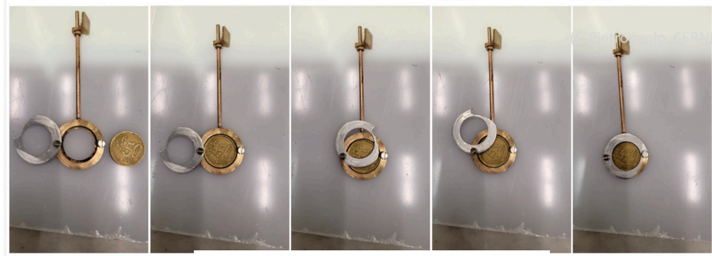
Bi207 source installation sequence
