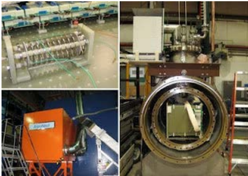
ArgoNeut TPC field cage and installation in NUMI underground lab. Will be moved to MCenter.
