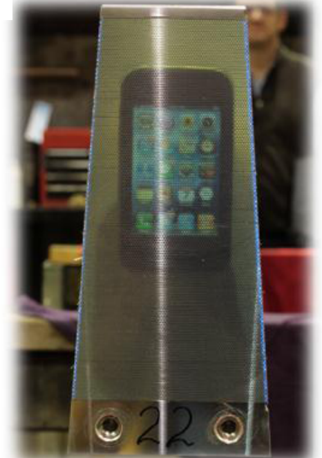
Polished BCAL module demonstrating optical clarity with cell phone held to opposite end
