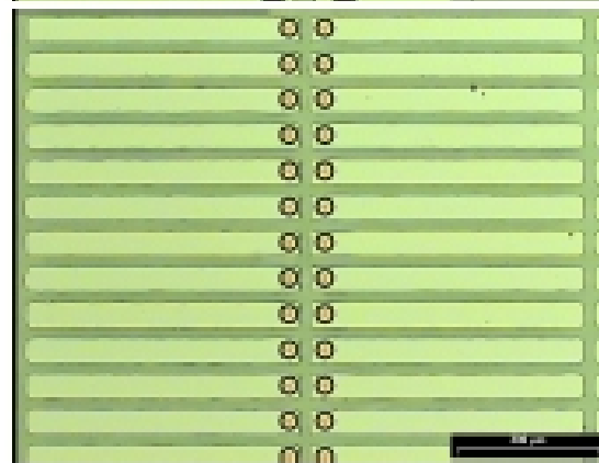
result after pixel metallisation patterning
