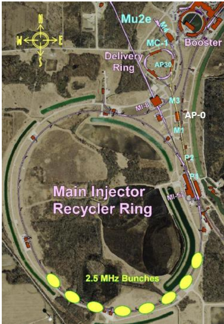
Figure 2 - Representation of bunches formed in the Recycler to be sent to Muon Campus
