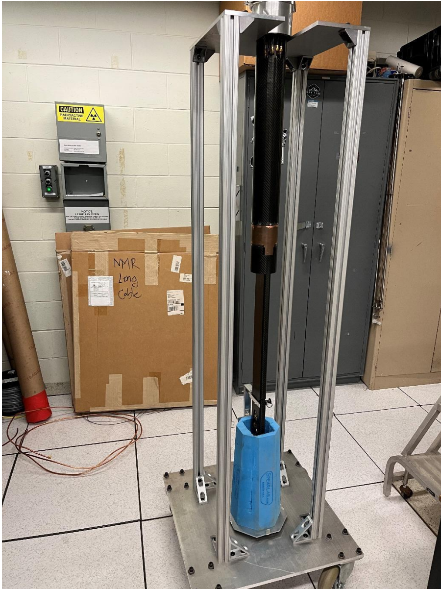
Figure 1 Target insert on the target transfer rack, the bottom of the target insert is in the transfer dewar with the dewar holder attached.
