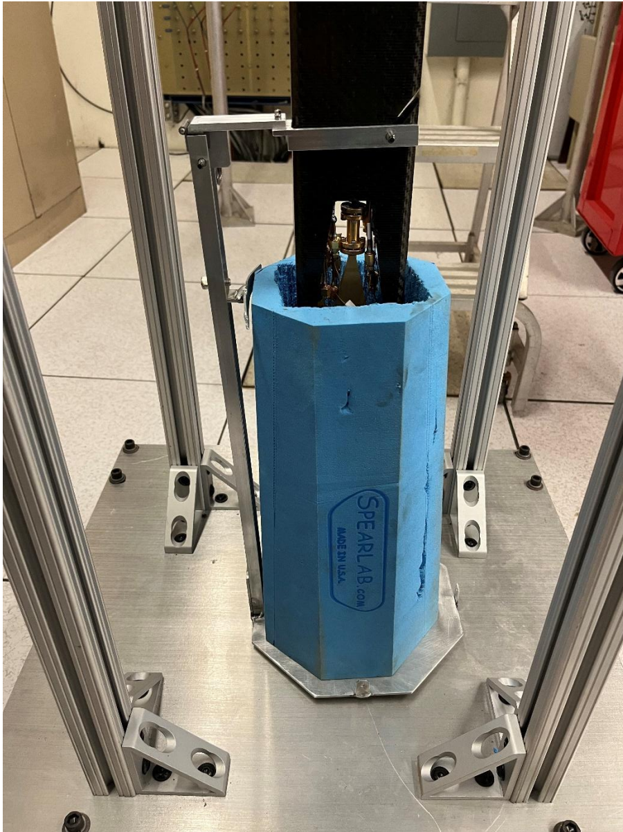
Figure 2 Target transfer dewar attached to the target insert using the dewar holder.
