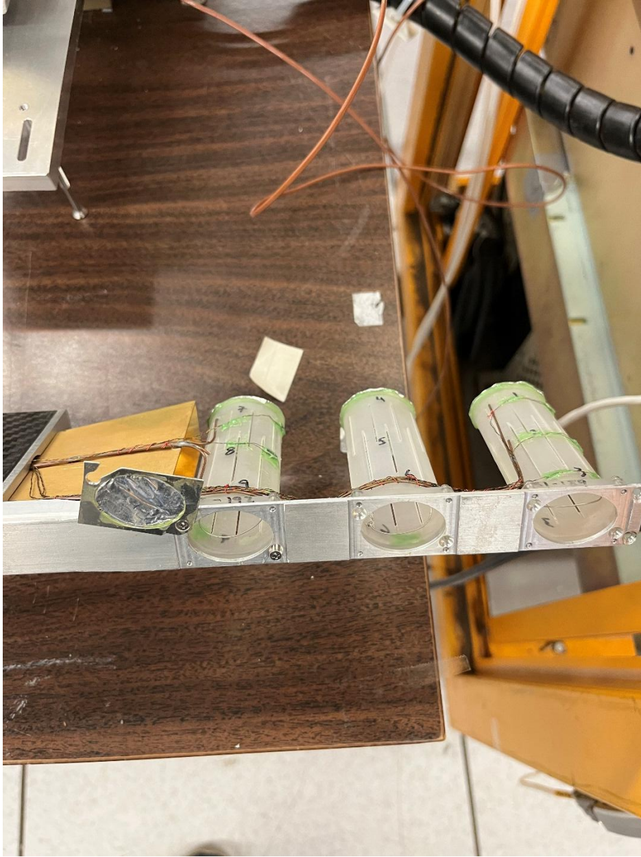
Figure 2 Target cut with cover opened. In the picture only one cup cover is shown, but all three cups will have covers.
