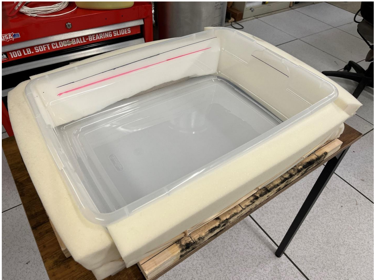
Figure 4 New LN2 tub sitting on top of the work desk. The black line indicates the fill level, the red line indicates the minimum level.
