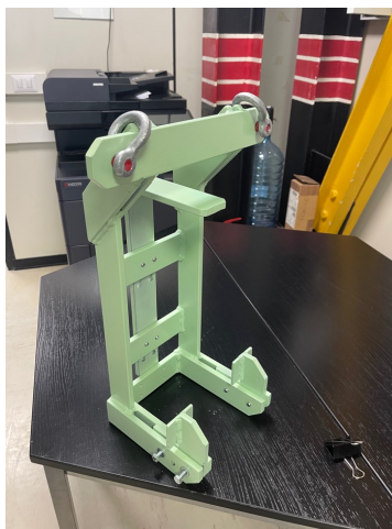
Special tool for dismounting the smallest module built and ready.
