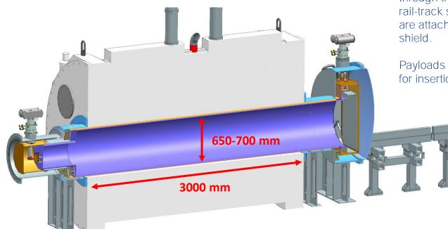
Payload can be inserted into bore through the side access hatch using a rail-track system. Rails (not shown here) are attached to the inside of the PT2 shield.
