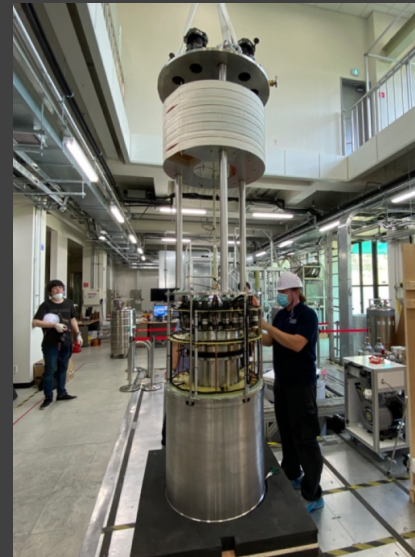
12 Tesla SC magnet 320mm bore diameter
