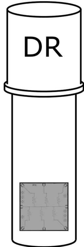
Vary  $\gamma$  dose at sample by adjusting distance
