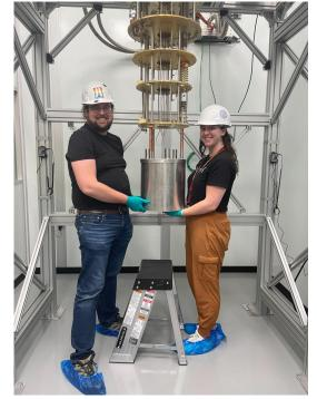
Significant volume above shield at base temperature for circulators and other magnetic components.
