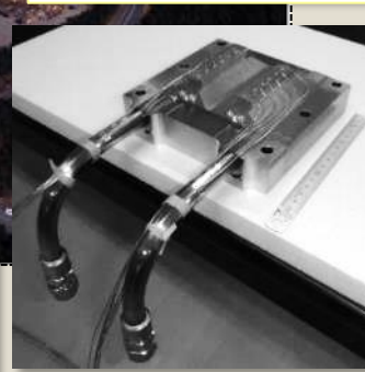
Hadron [HEF] Water cooled gold/ high-Z rotating target
