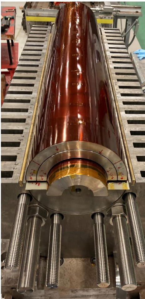
Coil block on the mirror
