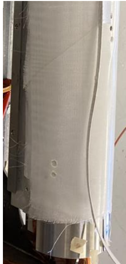
VT placed inside interlayer insulation
