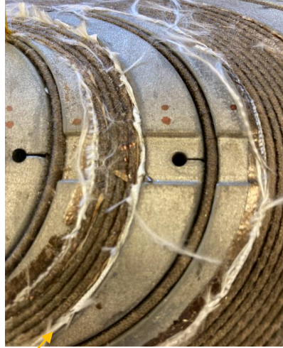
Coil OD after reaction
