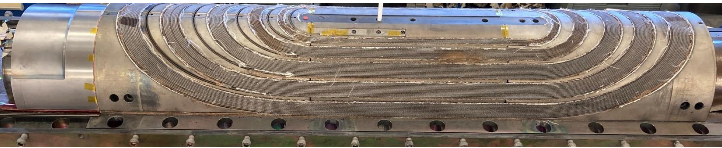
SMCT coil after reaction
