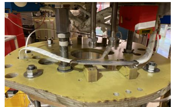
Current lead splicing
