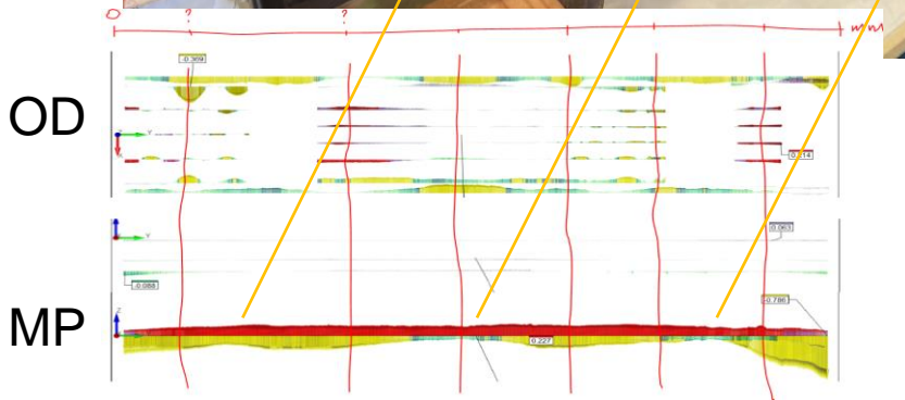
Correlation of coil size variation and tooling block position
