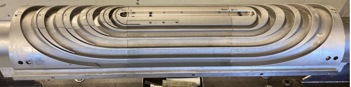
Coil outer layer mandrel before winding
