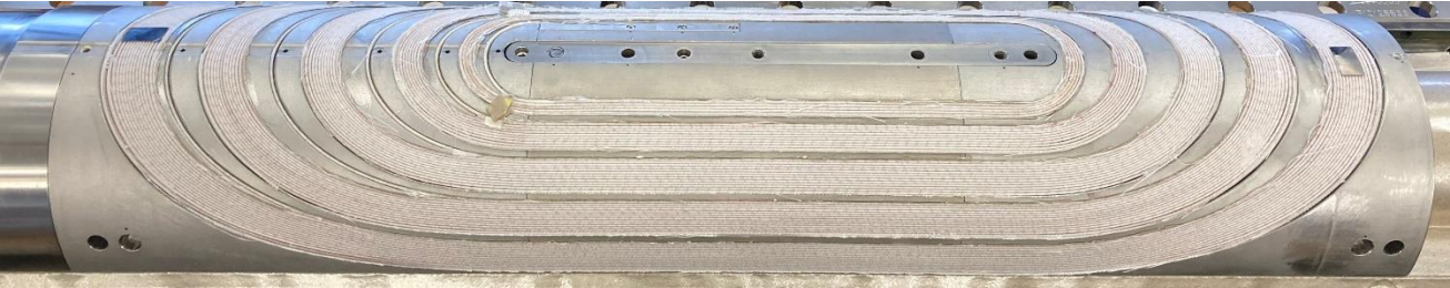
Completed outer layer winding
