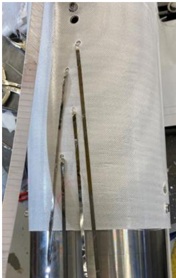
VT placed inside interlayer insulation
