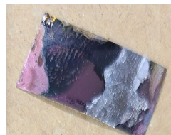
Delamination of YBCO layer
