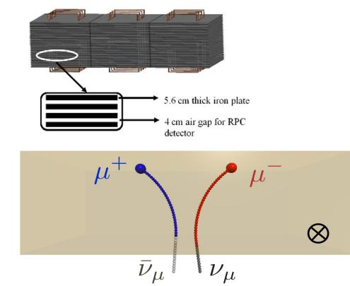
Resistive plate chamber (RPC) (active element) sandwiched between iron plates (passive element)
