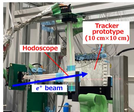
The setup of the beam test
