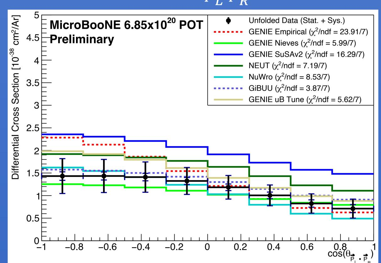
C. Opening angle between muon and proton sum
