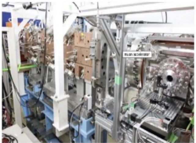
World first The experimental set up for muon cooling and acceleration at J-PARC. A beam of antimatter muons enters the apparatus from the right. Credit: J-PARC
