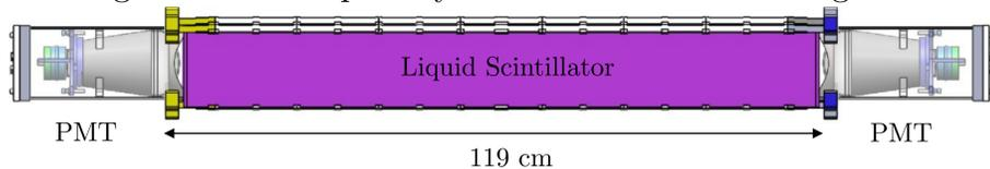
The ingress of liquid scintillator into PMTs led to the failure of some PMTs, resulting previous results to be dominated by statistical uncertainty.
