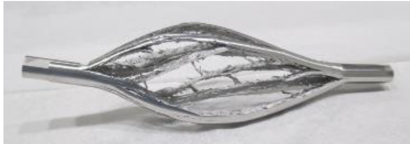
Thermal shock effect in an Iridium rod exposed to a high-intensity beam pulse at CERN's HiRadMat facility
