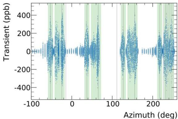
Electrostatic Quadrupoles transient field and NMR magnetometer.
