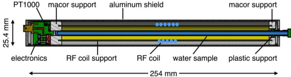
g-2 Calibration Probe Diagram.
