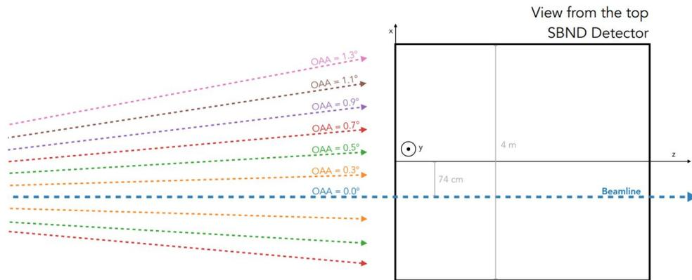
SBND positioned ~70 cm off beam axis and only 110m from target
