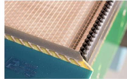
Field cage to ensure uniform electric field of 500 V/cm
