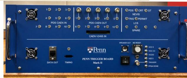
**Hardware trigger** primarily based on fast O(ns) PDS signals, also includes beam signals and CRT
