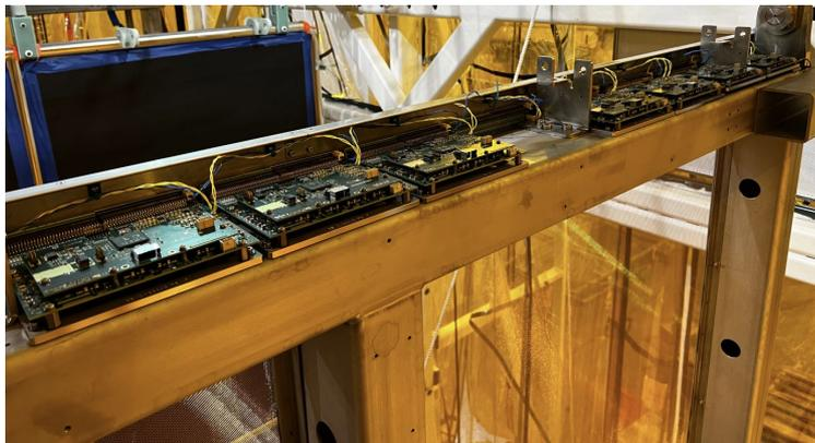
**TPC cold electronics** installed on anode plane frames
