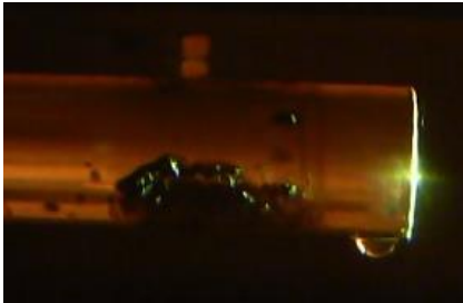
MINOS NT-01 target containment water leak (FNAL)
