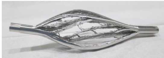
Test Iridium target irradiated at CERN's HiRadMat
